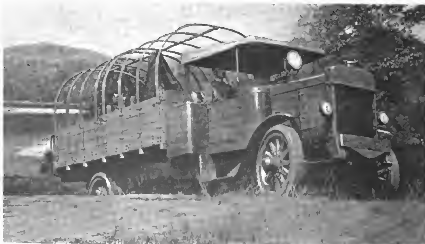
A complete truck climbing a difficult grade. Note the high radiator and hood, the searchlight mounted on the dash and the substantial bumper bar
